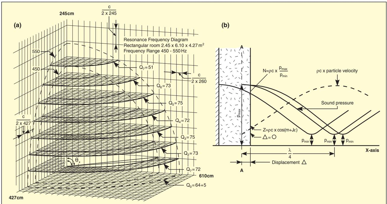
Figure 10. (a) Frequency of a standing wave in a rectangular room (distance from center) and the directivity. Rapid increase in numbers stems from increasing frequency. (b) Impact of standing wave on porous absorption material. From position at  $p_{min}$  and ratio  $p_{max}/p_{min}$ , complex acoustic impedance can be determined. Real impedance is found in Plane A-A.
