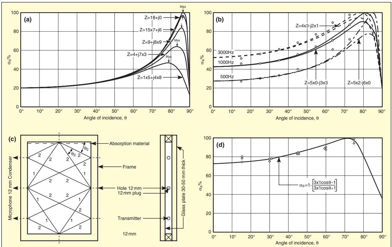
Figure 11. (a) Solid curves are F. V. Hunt's theoretical curves for increase of absorption with angle of incidence. (b) Dots are measured results made by Hunt in 1935 and measurements made at Chalmers in 1944. (c) Two 30-mm glass plates form a very flat room. A slow gliding tone excited resonances of standing waves in the enclosure. (d) Absorption for angles between 75° and 90° could not be experimentally verified.
