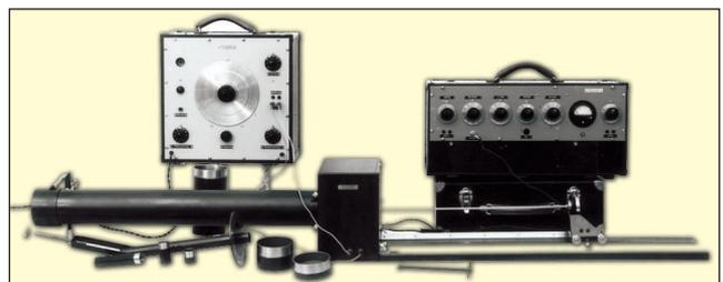
Figure 7. Beat-frequency oscillator (left) and line-powered frequency analyzer with two selective sections (six variable resistors and  $8 \times 6$  fixed capacitors). Standing-wave tube (front). All were made at the army's workshop in Ryvangen in 1942 and were beautifully crafted.
