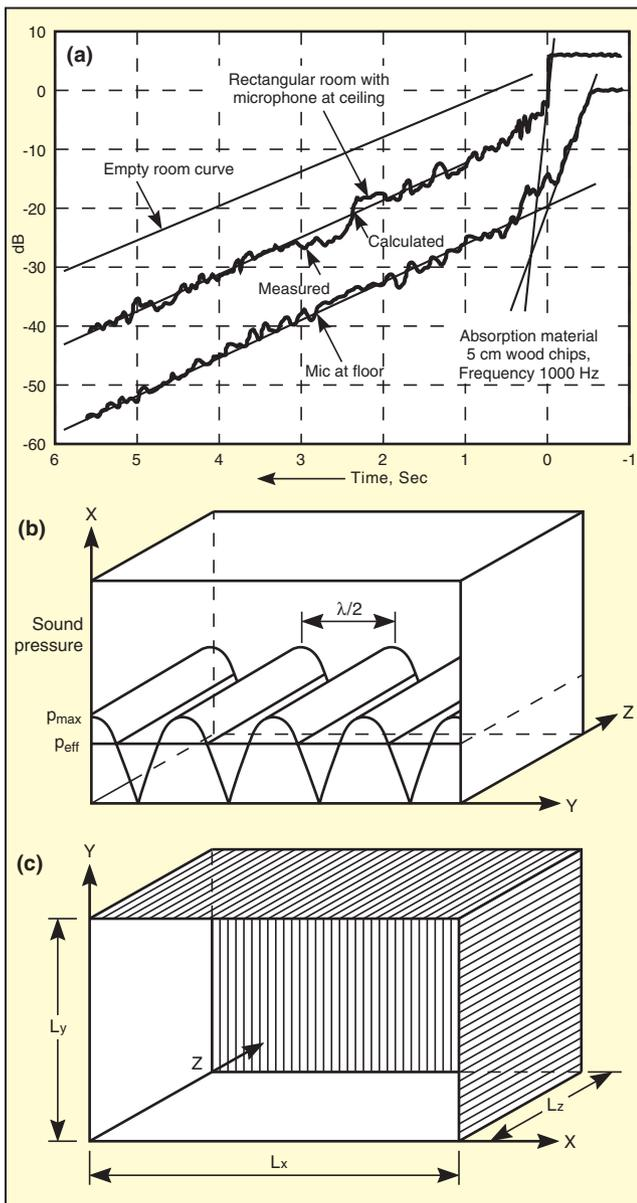
Figure 4. (a) Reverberation curves recorded with Nielsens's level recorder; note the detail. (b) Standing wave moving parallel to absorbing material covering the floor in a  $6 \times 6 \times 4$  m concrete room. (c) Only rectangular rooms, where each wall section has the same acoustic impedance, can be calculated by solving the wave equation.
