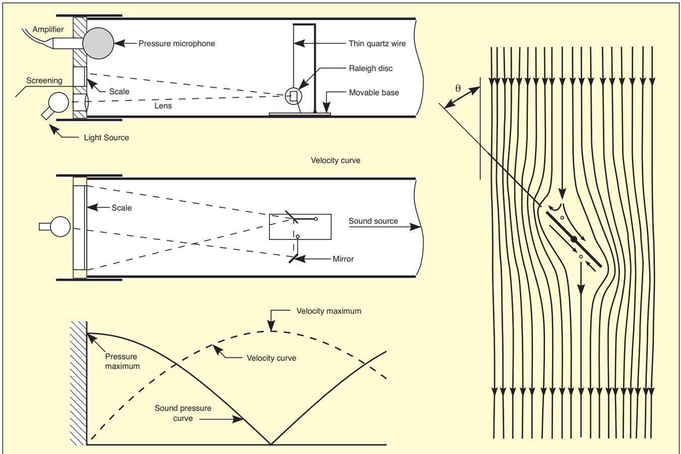
Figure 8. J. Oskar Nielsen's setup for calibration of standard microphones by using a Rayleigh disk. He obtained an accuracy of  $\pm 0.2$  dB; but one must correct for both the thickness of the disk and temperature.
