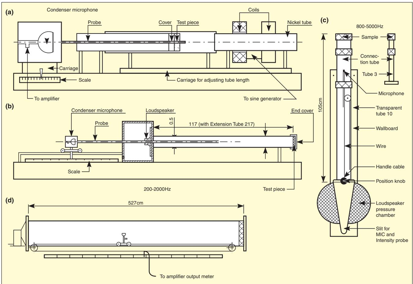
Figure 2. (a) Standing wave tube (SWT) for measuring acoustic impedance at high frequencies, made at LTT around 1930. (b) Later model was in production at B&K for more than 40 years. (c) Newer vertical SWT covering frequency range 100 Hz to 5 kHz with two tube diameters: 10 cm and 3 cm and movable 6-mm microphone. (d) Older LTT tube developed by V. Jordan.
