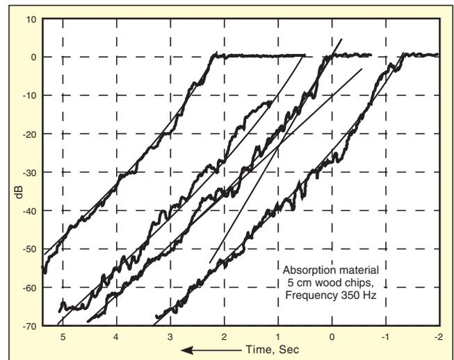
Figure 5. Reverberation decay times in the same room as Figure 4 at lower frequencies; flutter echo less pronounced. With longer wavelengths, absorption material has better contact with parallel sound waves. That is one reason why flutter echoes are a high-frequency problem.
