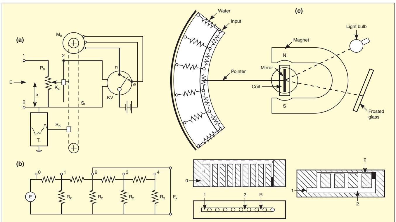
Figure 3. Jens Oskar Nielsen's logarithmic potentiometer is a chain of T-link resistors, where the resistive medium is water. (a) Principle of the writing logarithmic potentiometer. (b) Some of Nielsen's original drawings. (c) Practical construction of level recorder, with a moving coil element, and pointer tip that dips into the water potentiometer. Total dynamic range can be changed by changing the water level.
