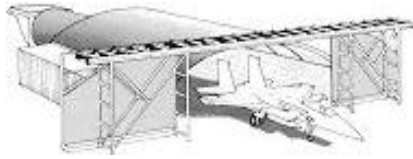
Figure 24. "Hush-house", designed to confine the noise of jet engine tune-ups.
